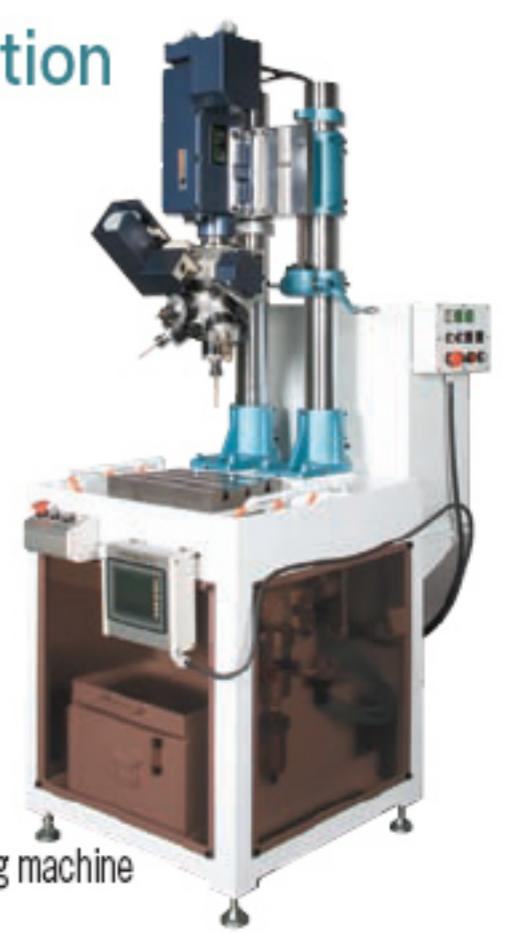
Automatic drilling machine utilizing 4TH3S
